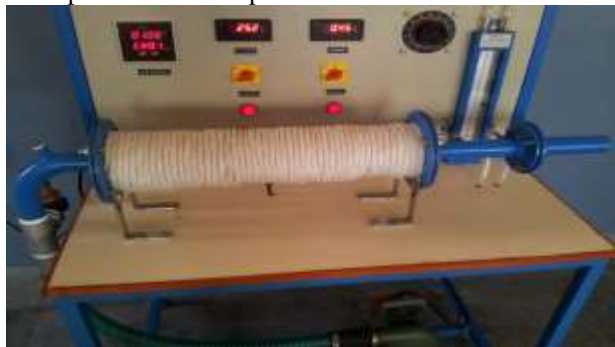
Fig. 3.1 Experimental Set Up Of Forced Convection
